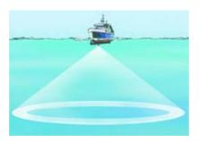
An Omni transmission means that the sound is transmitted in a full 360 degrees circle around the vessel, while Sector means that it is transmitted in a defined direction shaped like a cone. The Sector transmission will provide you with a longer range.
