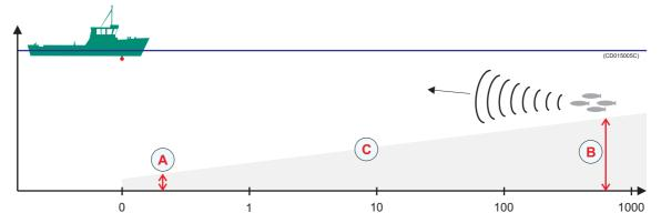
The drawing illustrates the TVG principle: The gain at time (B) is larger than at time (A).
