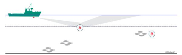
If you transmit a sonar beam down towards a temperature or salinity layer (A), it will be reflected as indicated in the illustration. The school of fish (B) you thought you would see will not be visible at all.
