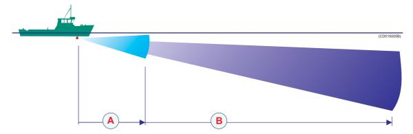
(A) = Wide beam, (B) = Narrow beam (Normal)
