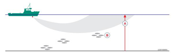
When the temperature decreases (A) closer to the surface, the sonar beam is deflected up as indicated by the illustration. The school of fish (B) you thought you would see is once again not visible at all, and you will also see a ring of surface echoes.
