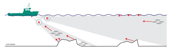
The echoes from the bottom will vary with how uneven the bottom is, what kind of bottom you have under your vessel, (rock, mud, sand etc.) as well as your current tilt setting. The echo from the sea surface will vary with the current sea state and your current tilt setting.
